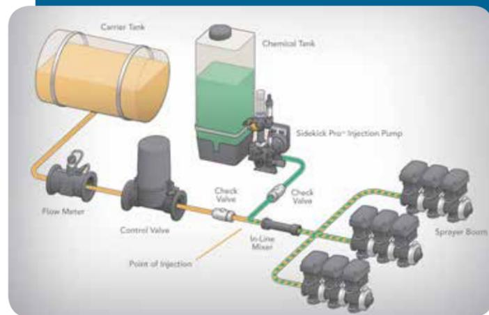
It's the direct injection system that sets a new standard for chemical applications of every type, with unprecedented precision, savings and safety. No tank mixing required —and with the industry's first remote and closed calibration and prime feature, you're ready to go in minutes. It also features:
