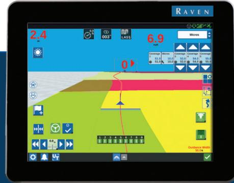
The CR12 is the latest field computer in the CRX display family, joining the CR7. Uniquely, the CR12 offers an extensive field planning feature, allowing the user to define AB-lines and reference lines of the field boundary. The user can then setup the complete field, including multiple headlands, spray tracks, greening zones and tracks with different working widths.
