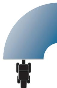
The outer end of the boom can travel up to three times the speed of the machine or inside of the boom when turning.
